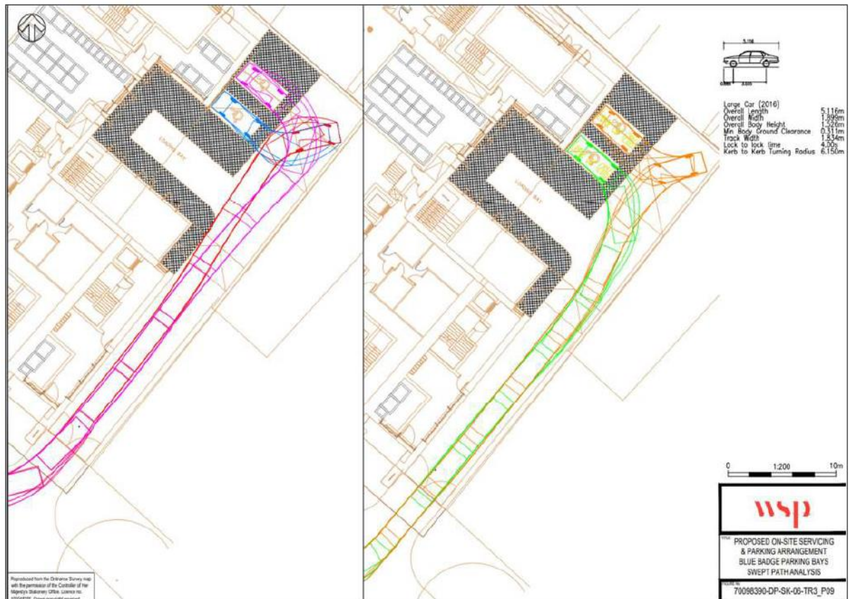
Image (above): On-site servicing and parking arrangements
